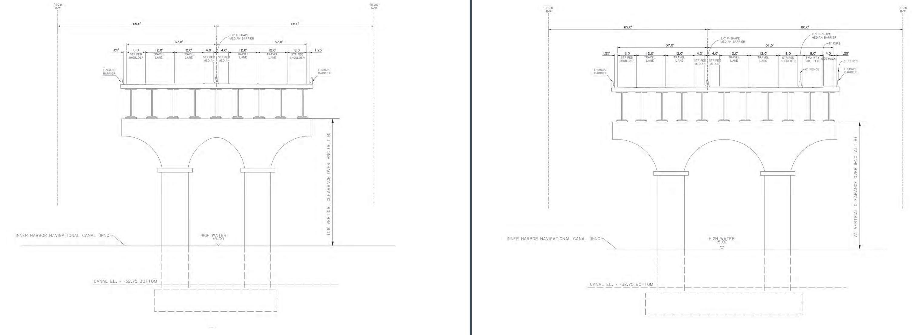
Mid-level Movable Bridge **Double-leaf Bascule Bridge 73 Foot Vertical Clearance**
